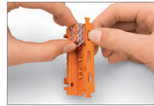
Removing connector from the mounting carrier
